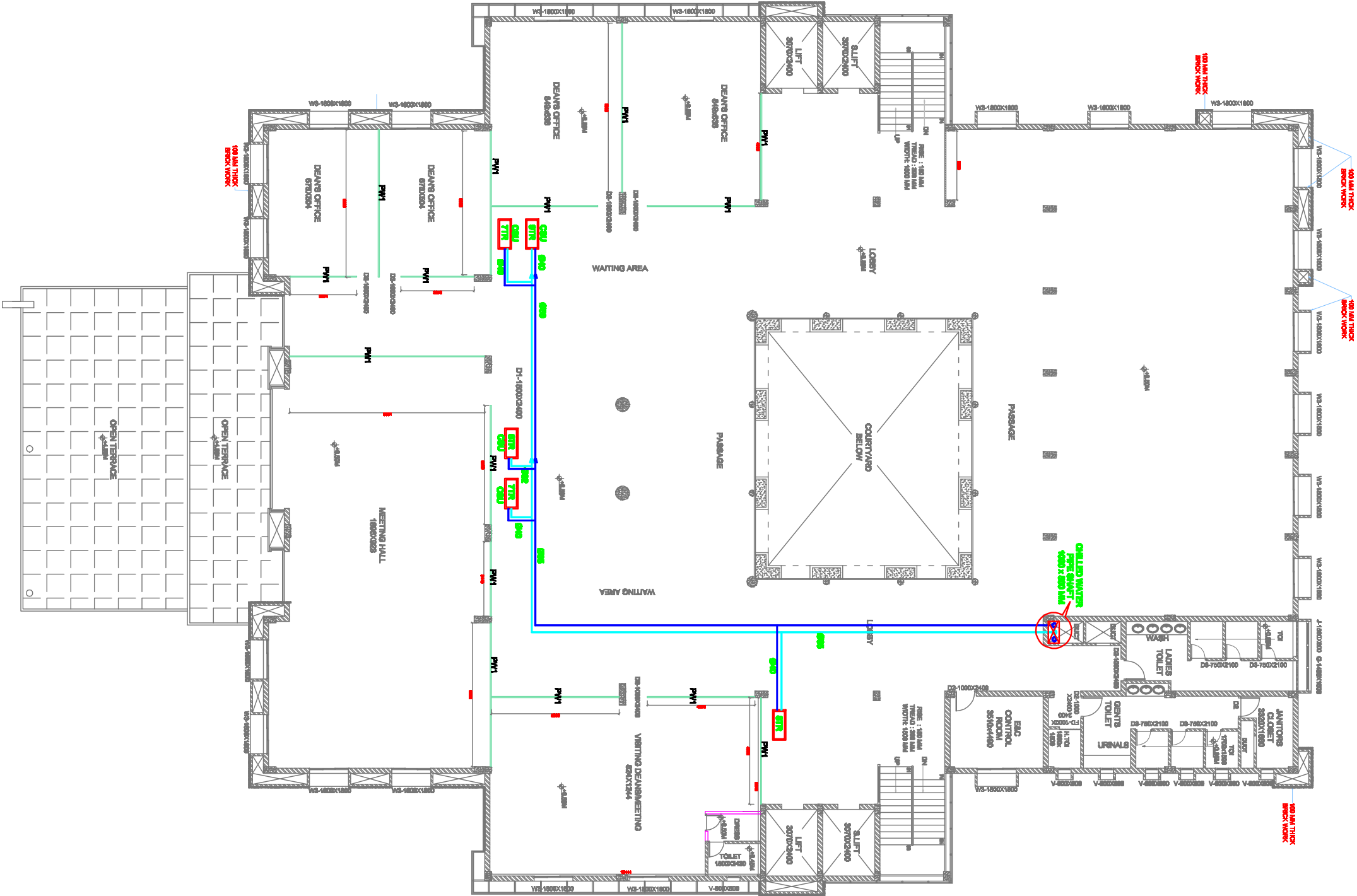
AHU & CHILLED WATER PIPE LAYOUT FOR SECOND FLOOR
