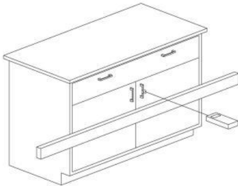
Figure 8. Base Cabinet Door and Drawer Pull Horizontal Load Test Configuration
