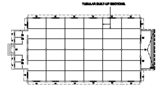
PLAN SHOWING POSITIONING OF TUBULAR BUILT-UP SECTIONS.
